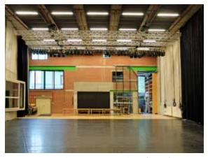
Wooden sprung floor with a total surface of about 14m x 20m, maximal load  $500 kg/m^2$ .
